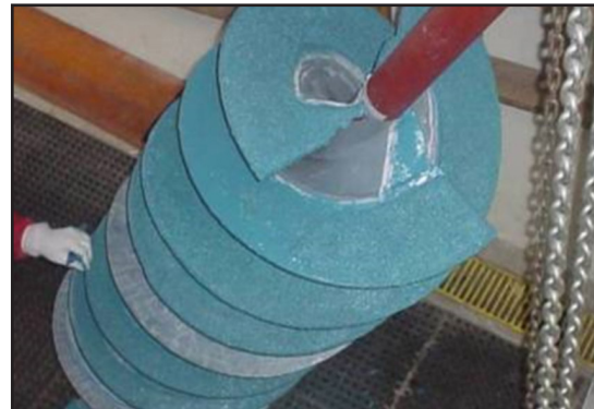
Screw during ARC MX1 coating process
